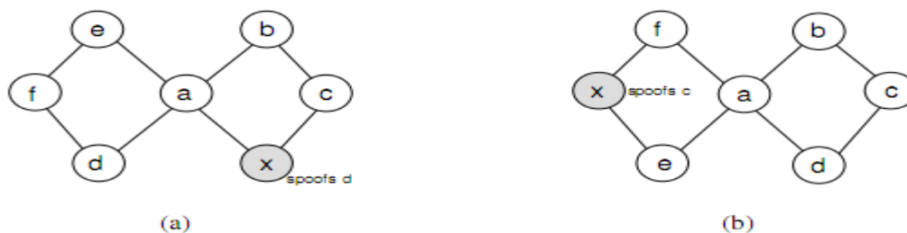
Fig 2.(a) flooding disruption attack due to link spoofing and (b) flooding disruption attack due to the malicious node.
